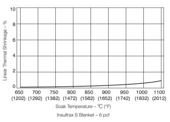
\*Shrinkage Test Performed at Soak Temperatures for 24 Hours.
